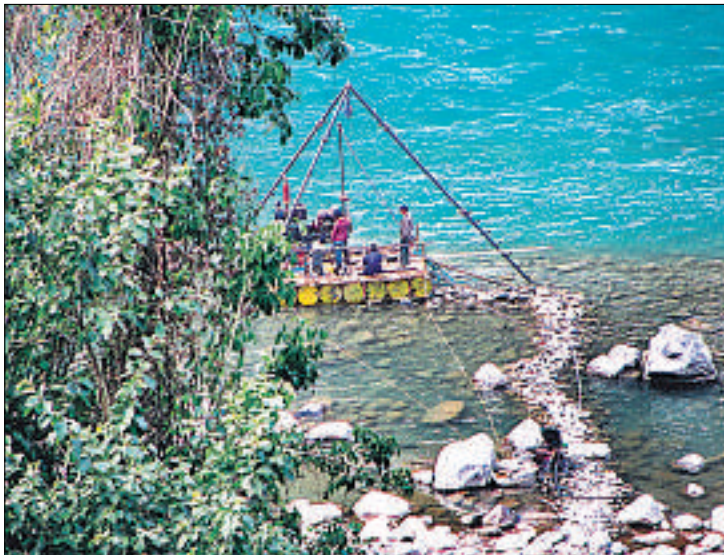
■ Officials test the quality of soil and rock as part of a plan to construct hydel projects on Lohit river in Arunachal Pradesh. NIVEDITA KHANDEKAR/ HT PHOTO
